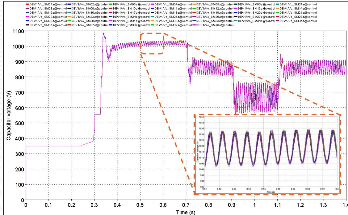
Developing modulation and control schemes for our MMC-based STATCOM involved the complex task of instantiating and connecting numerous submodules in each upper and lower arm across all three phases.
